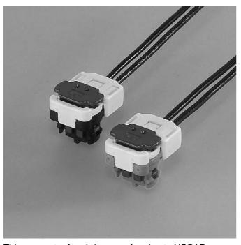
This connector for air-bag, conforming to USCAR standard, has intelligent CPA, which allows locking the connector, incomplete mating detection and release of short-circuit at the same time.
